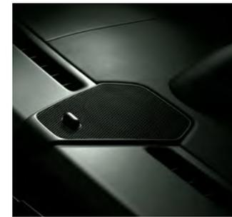
A 2.75-inch (7-cm) midrange centerfill speaker in the instrument panel
