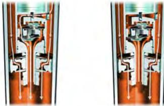
Left: Rebound in Normal mode—bypass valve open
