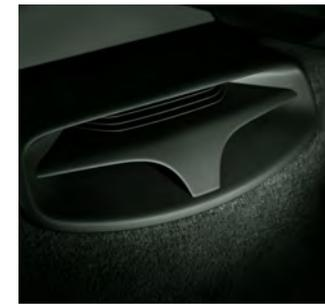
One 4 x 6-inch (10 x 15-cm) woofer in a 5.8-liter custom-engineered bass enclosure with a two-state modulation amplifier in the center console on the passenger side
